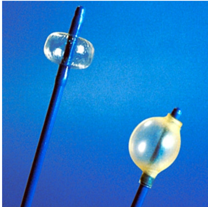
PHOTO 8. On the left is a high pressure, thin walled balloon. On the right is an elastic latex balloon. Elastomeric balloons often unintentionally expand asymmetrically as seen here.
