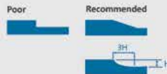
Fig. 1.2 Illustration of inside & outside draft angle to allow easy component removal from tool.
