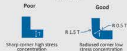
Fig. 1.7 Design considerations for radii for MIM processing.
