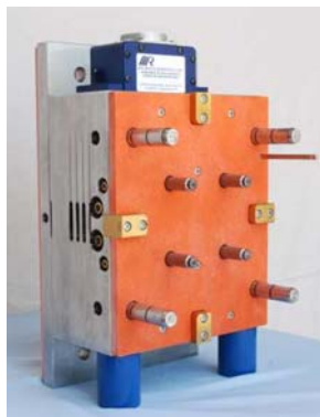
Figure 13: Typical cold runner system for LSR molding [15]
